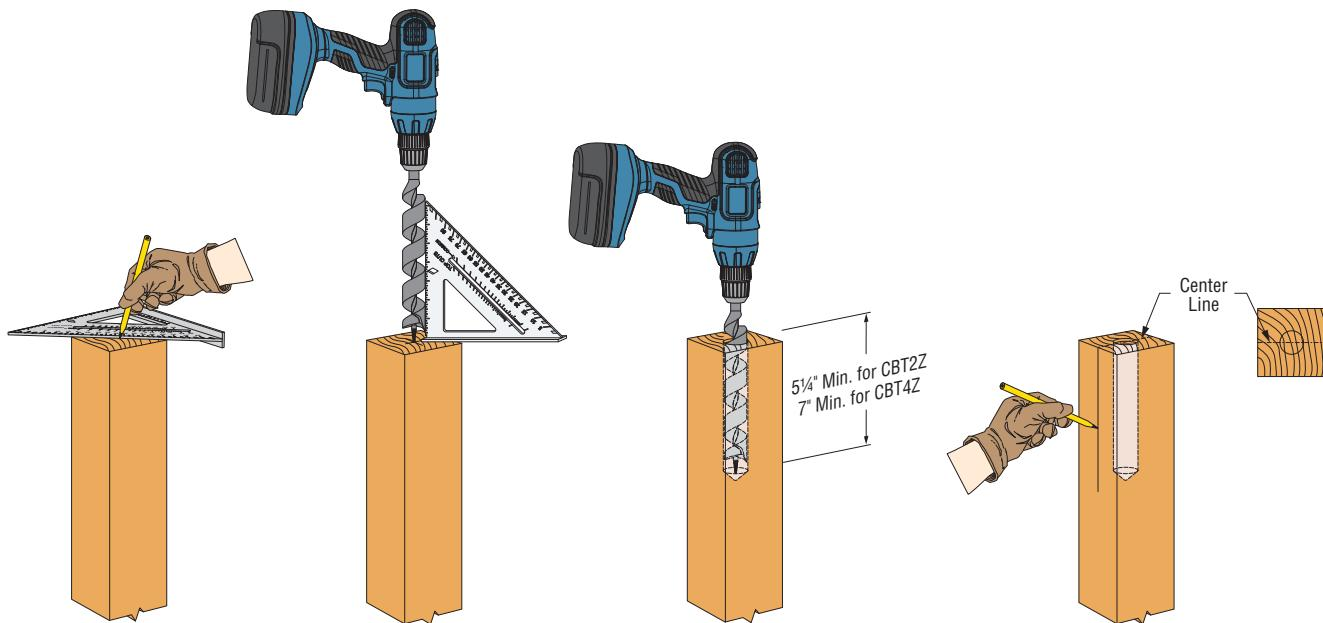
1. On a squared-off post, mark the center of the top of the post.
