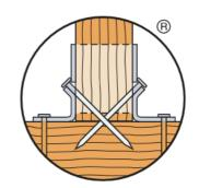
Double-shear nailing shall use minimum 2½"-long nails or 2½"-long SD screws
