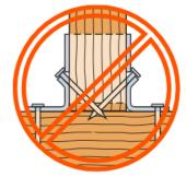
Shorter fasteners may not be used as double-shear nails
