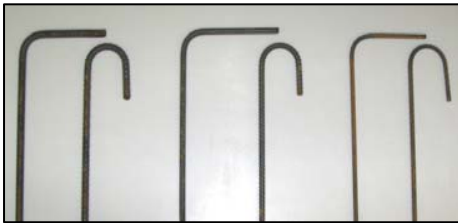
Benner-Nawman, Inc. Part # MBC-16B Bending roller dia.: 2.5"
